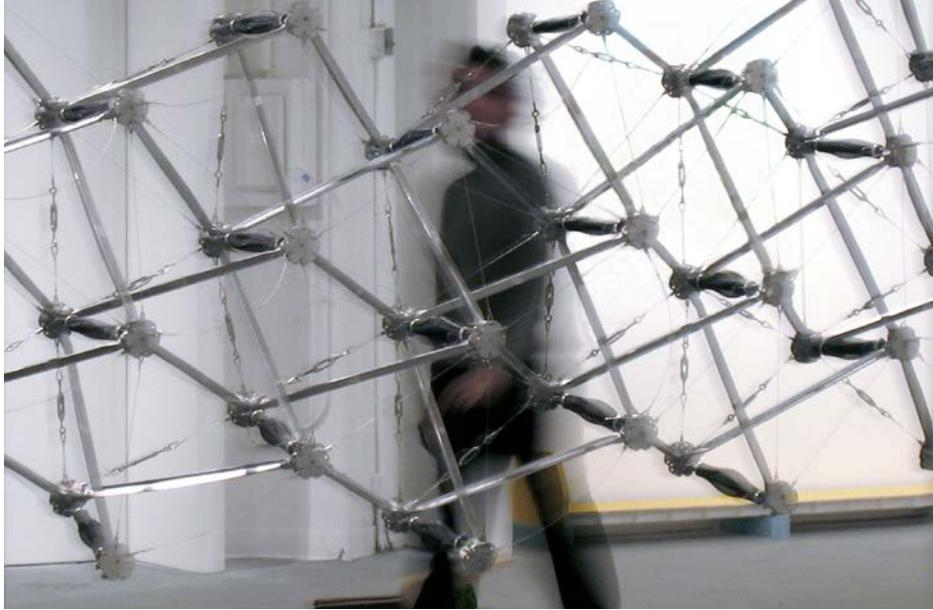
6) A reduced scale cast aluminium prototype of a mixed class one & four, actuated tensegrity structure with NiTi thermal memory actuators, built by the author. This work was most recently recognized in:
