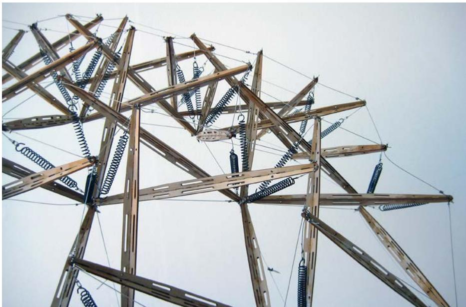
7) An early working prototype for a class two actuated tensegrity tower built by the author. This photograph depicts an early instrumentation that has been generalized and advanced since. This work was most recently recognized by:
